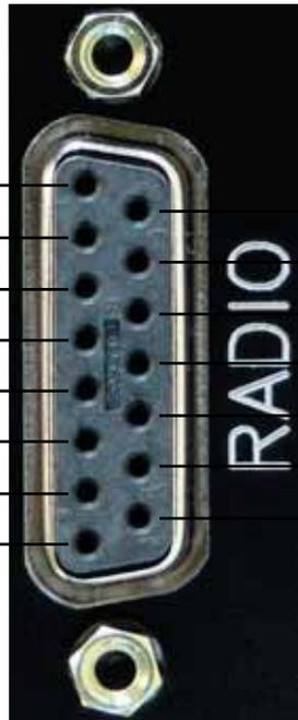
Both sockets have an identical pin out. The lower one connects to radio 1 and provides I/O 1 - 4, the upper one to radio 2. and provides I/O 5 - 8.
