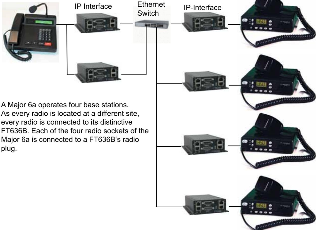
A Major 6a operates four base stations. As every radio is located at a different site, every radio is connected to its distinctive FT636B. Each of the four radio sockets of the Major 6a is connected to a FT636B's radio plug.
