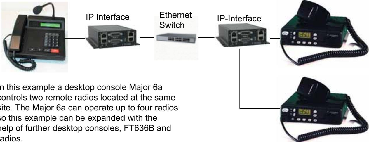
In this example a desktop console Major 6a controls two remote radios located at the same site. The Major 6a can operate up to four radios so this example can be expanded with the help of further desktop consoles, FT636B and radios.
